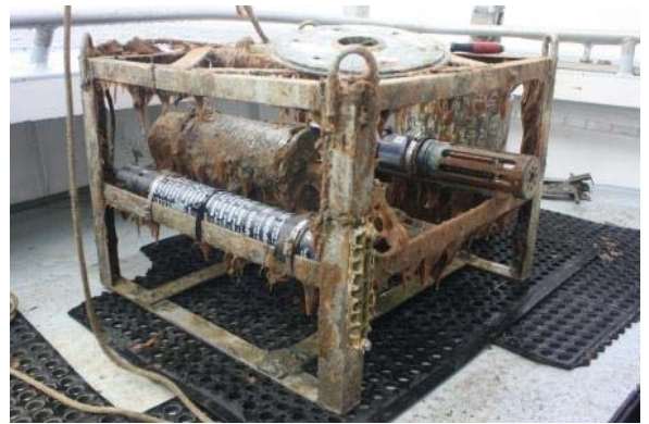
The CBIBS Gooses Reef bottom water-quality sensor tracks parameters including dissolved oxygen nearly 40 feet below the surface.
